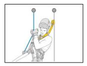
The ASAP'SORBER allows the rope to be kept at a distance, to protect it during certain work phases.
